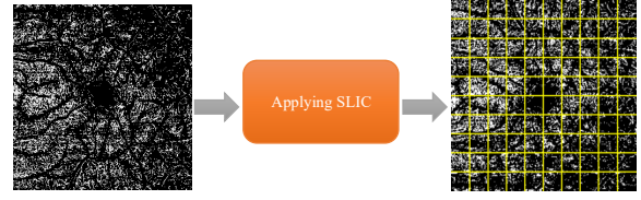
Fig. 5. Applying SLIC, to segment OCTA image into 100 super-pixel.
