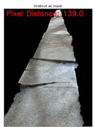
The ultimate goal is to get the measurements of the horizontal and vertical displacements on the sidewalk. Once we find the pixel distance for the x and y displacements, we convert it to centimeters. Those measurements will be used as part of the parameters in labeling the priority of the sidewalk images.
