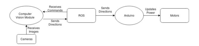
This is a diagram of how the computer vision module will help drive commands deciphered from detected objects, which will call different states within ROS.
