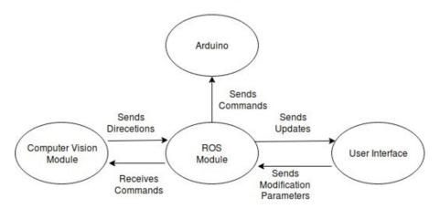
This is a diagram of a ROS module, and how it sends and receives messages from different parts of the platform.
