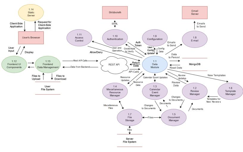
The overall system was split into three categories of modules: frontend modules that run on the client side, backend modules running on the server, and a static server to serve the client-side code. This distinction was made to simplify development: the frontend and backend can be developed simultaneously with relative ease once the REST API has been specified.
